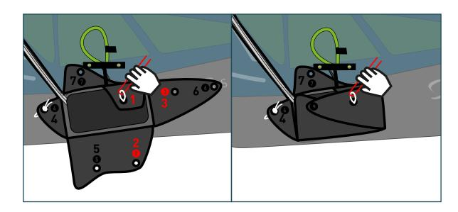
Push the yellow right plastic pin through the loop to fasten and secure the assembly. Remove the pin.
