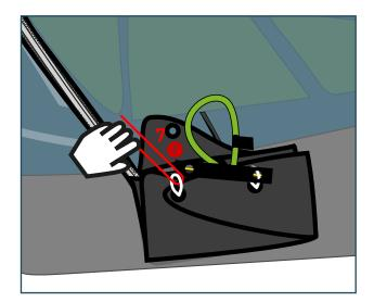
7 Close the risers zipper sleeve by pulling the tab to the end then back to the beginning
